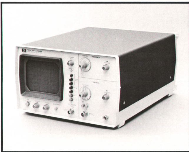
Fig. 2. Lower-priced Model 1221A Oscilloscope is identical to Model 1220A except that it has only one vertical channel.
